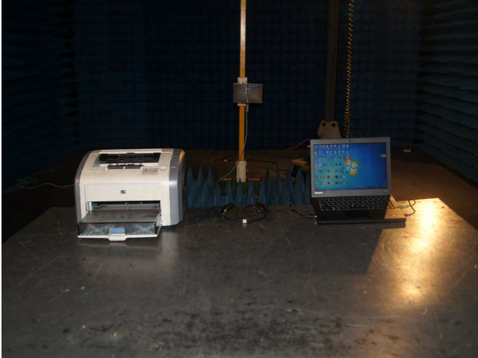
Photograph 7: Set-up for Radiated Emissions, above 1GHz
