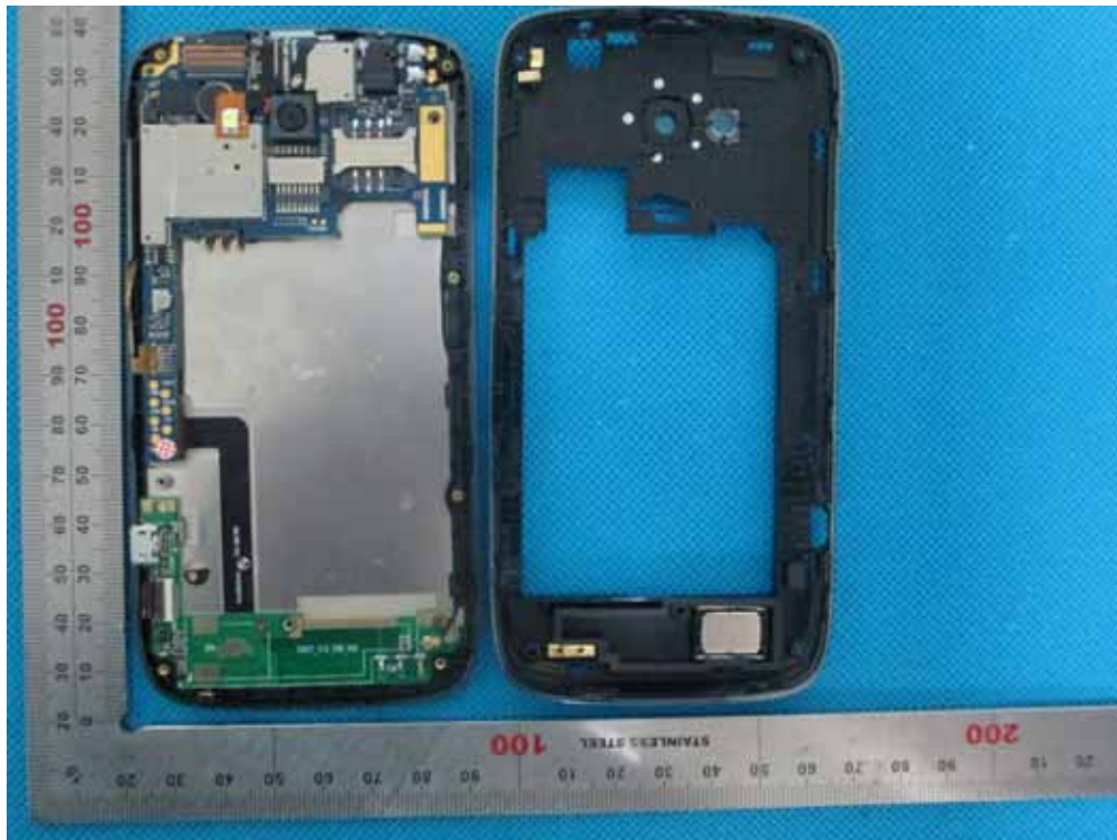
INTERNAL VIEW OF EUT-1
