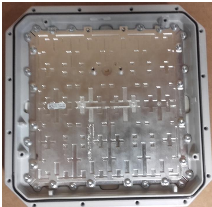
Figure 2: Antenna frame assembly showing antenna interface (Interior view)
