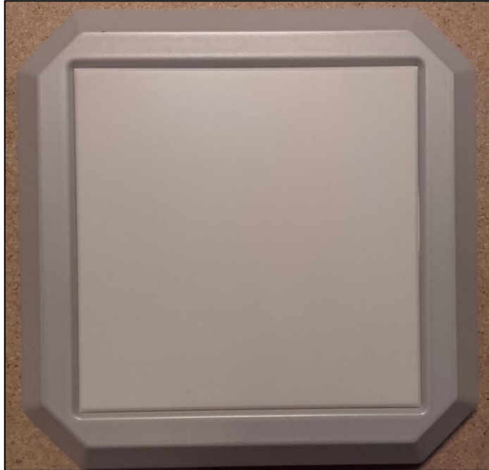
Figure 1: Antenna frame assembly showing Radome (Exterior view)
