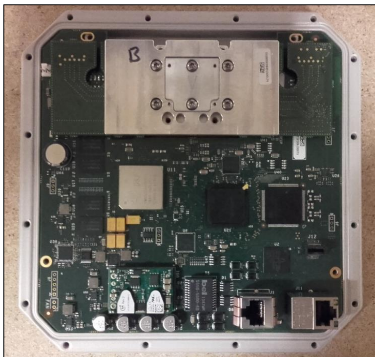
Figure 4: Assembled Unit less Rear Heatsink Plate
