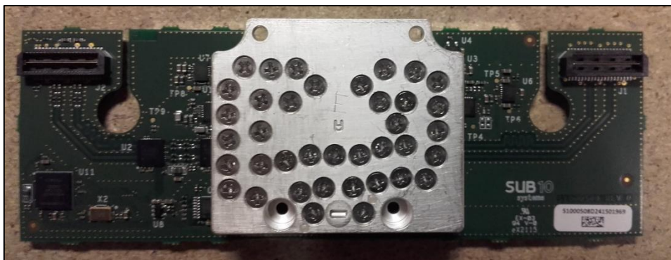
Figure 5: Microwave Unit Assembled with Control Board and Diplexer (Component Side)
