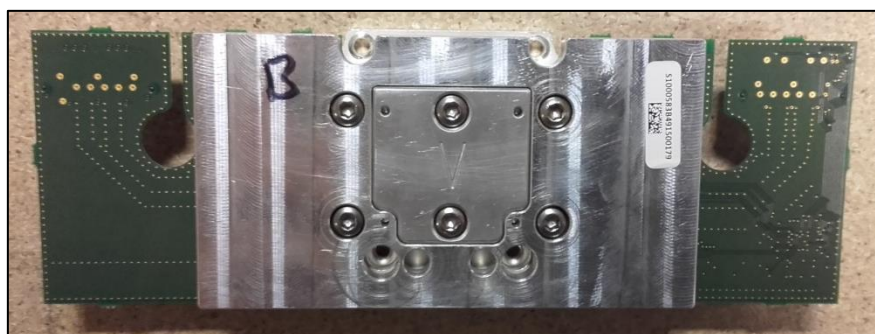
Figure 6: Microwave Unit Assembled with Control Board and Diplexer (Heatsink Side)
