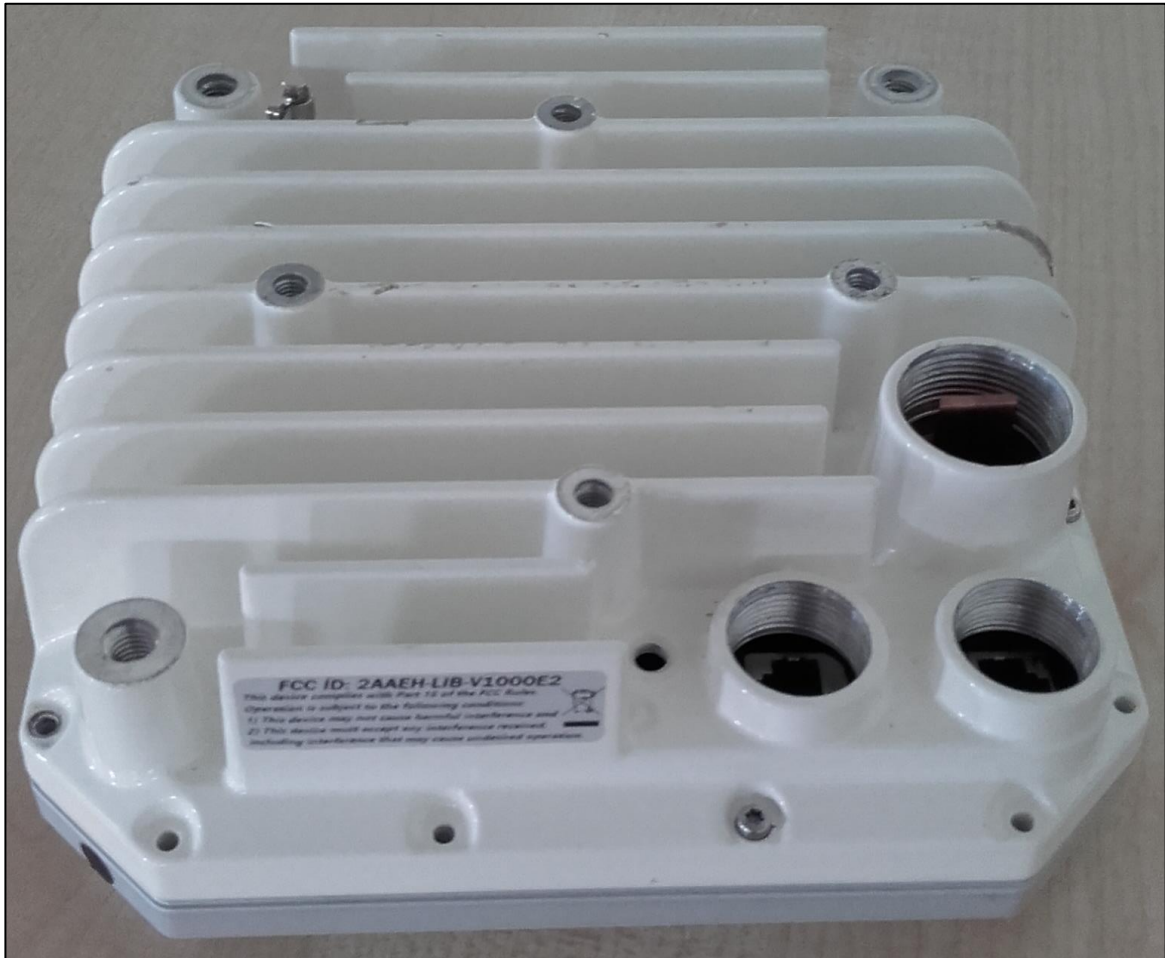
Figure 1: Rear view of Liberator-V1000 Dual-port showing polarization marking dot on antenna front frame, and FCC regulatory label
