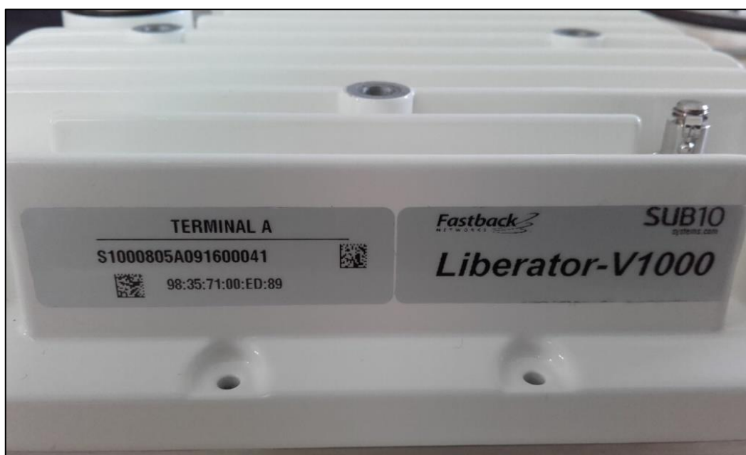
Figure 3: Close-up view of label with serial number, MAC address and QR code, and also model number label.
