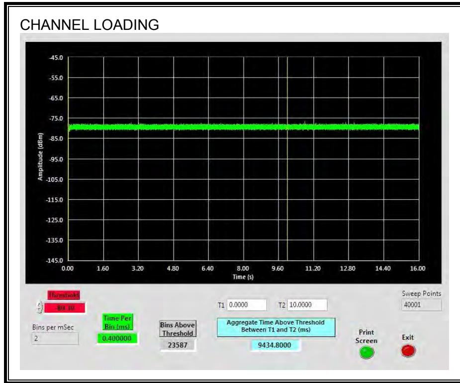
The level of traffic loading on the channel by the EUT is 94.34%
