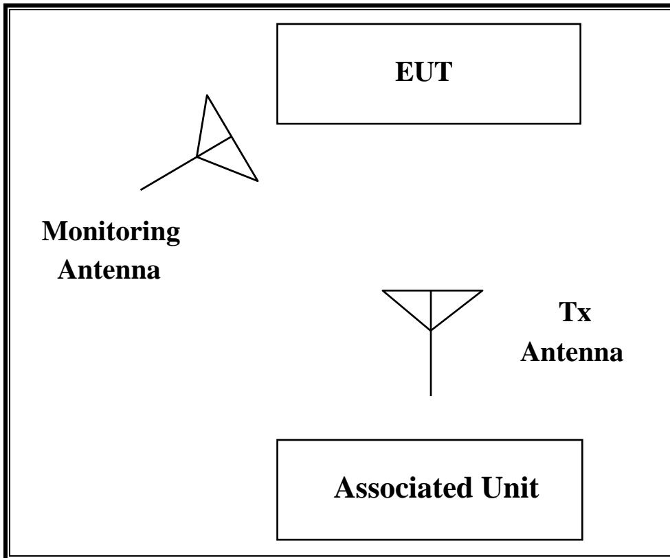
**Note:** Monitoring Configuration 2 was used during CAC testing.
