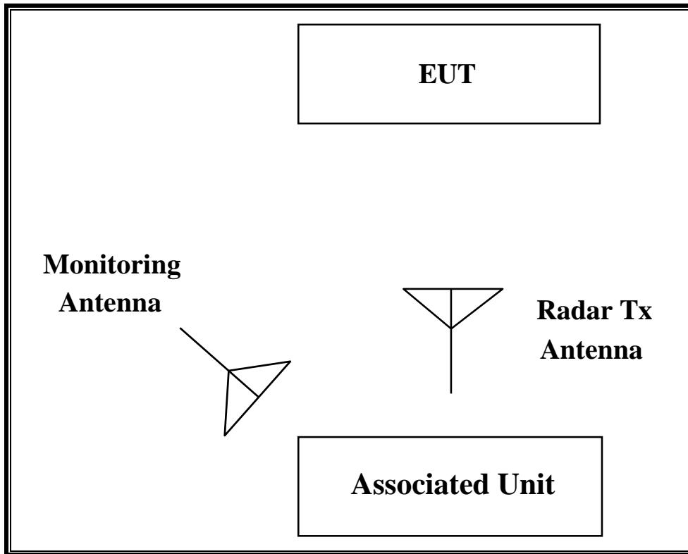
**Note:** Monitoring Configuration 1 was used during Traffic/Channel Loading, Channel Move/Aggregate Time and Non-Occupancy testing.
