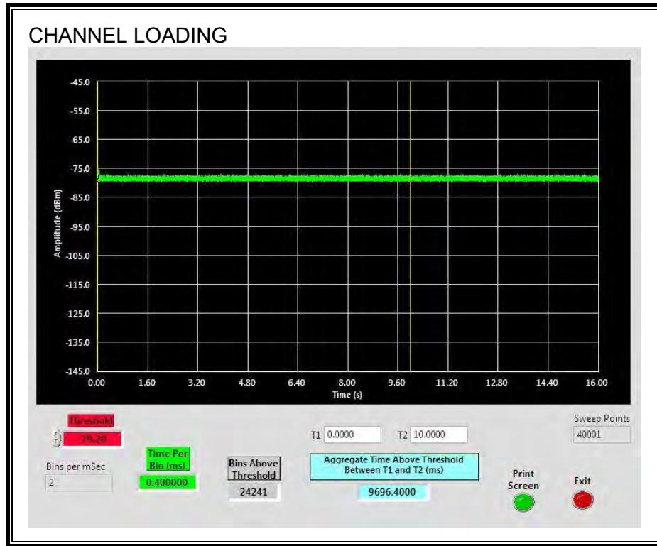
The level of traffic loading on the channel by the EUT is 96.86%.
