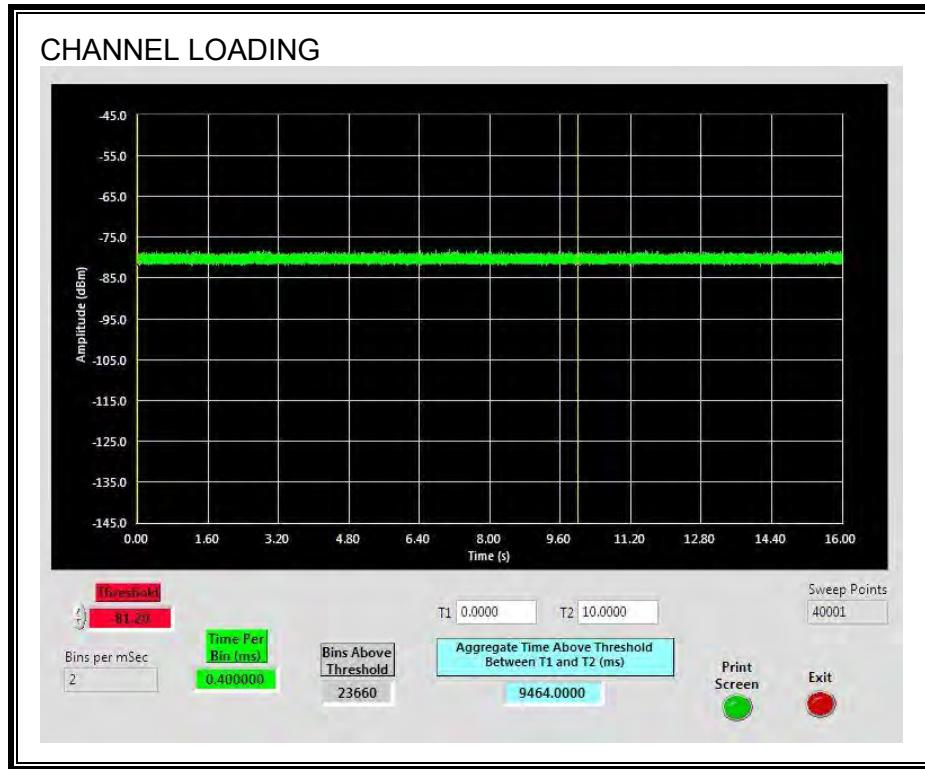
The level of traffic loading on the channel by the EUT is 94.64%
