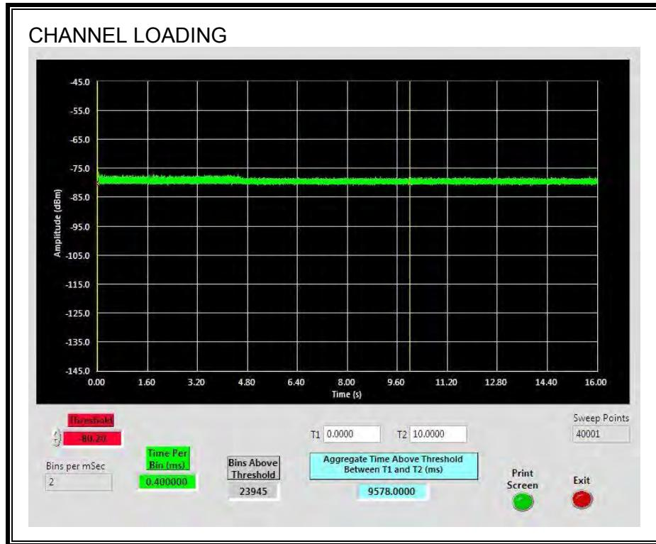
The level of traffic loading on the channel by the EUT is 95.78%
