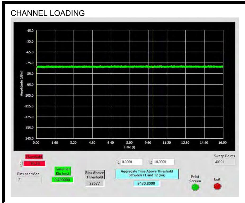
The level of traffic loading on the channel by the EUT is 94.3%
