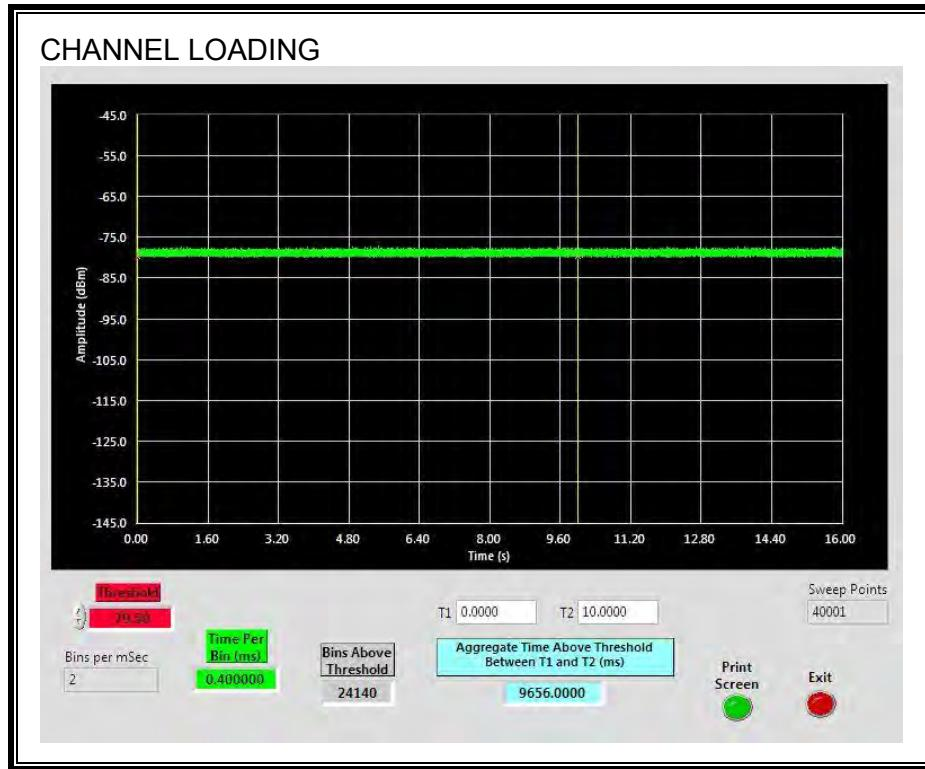
The level of traffic loading on the channel by the EUT is 96.56%
