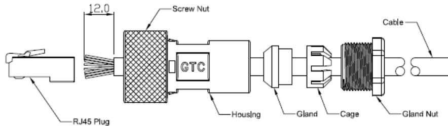
The connector will work with CAT5E and CAT6 cables and other cables having an outer diameter between 5.0 and 6.0 mm. NOTE: Use only weatherproof, shielded cable.
