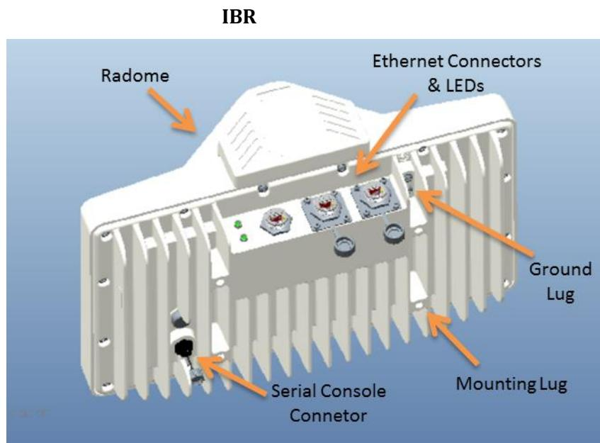
The Gigabit Ethernet port that is connected to the radio (not externally available) is identified as Gigabit Ethernet 3 (ge3). Radio parameters are configured through the radio 0 interface, while switching parameters that apply both to the physical Gigabit Ethernet ports and the radio port, such as VLAN, QoS, and CoS, are configured through the Gigabit Ethernet interface.
