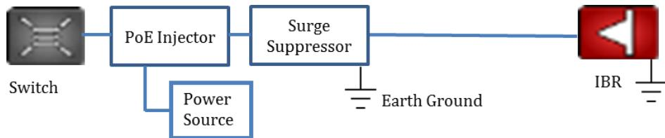
The surge suppressor should be installed ahead of the cable ingress to the enclosure or structure housing the switch in order to maximize protection to the switch. The surge suppressor should be connected to a true earth ground with materials that meet the manufacturer's specifications.
