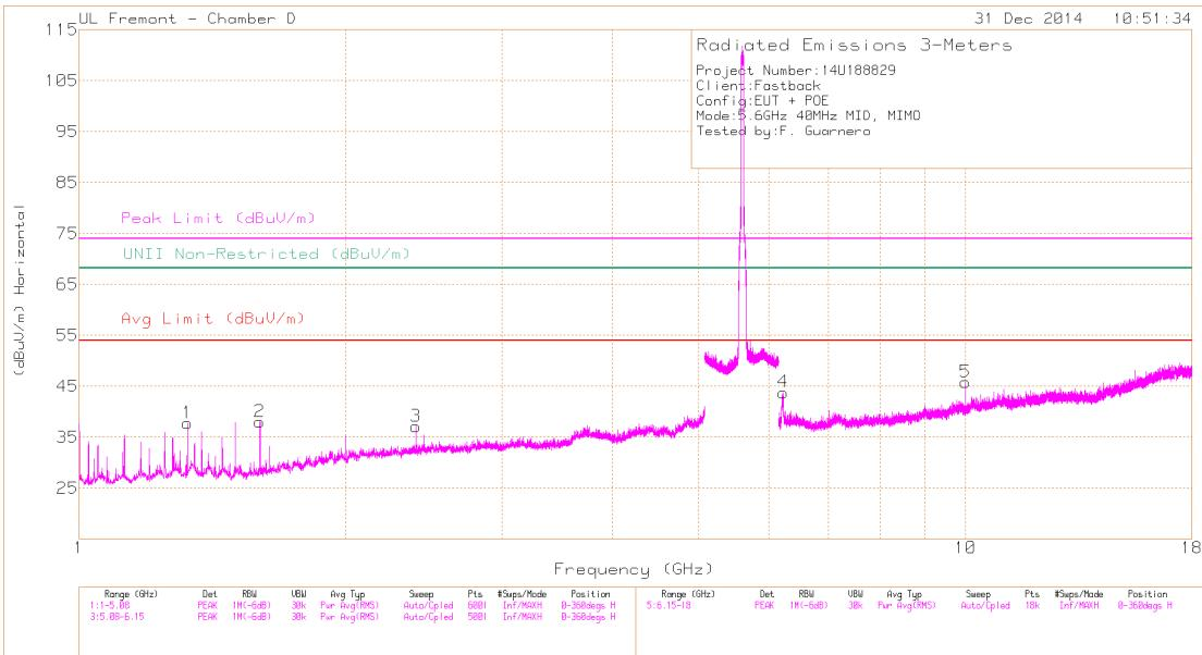
FCC Part15C All 5GHz UNII and DTS Spurious Emissions with Average Scan.TST 30915 24 Mar 2014
