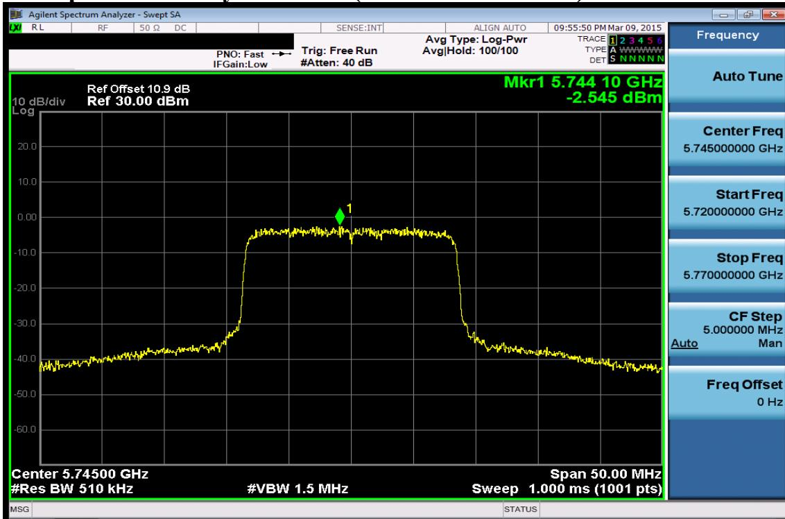
**Peak Power Spectral Density Data Plot (CH Mid 5785 MHz)**
