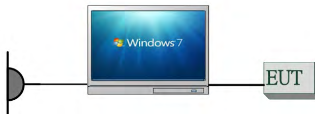
Fig. 2-2 Conducted Emission (AC Power Line) Configuration
