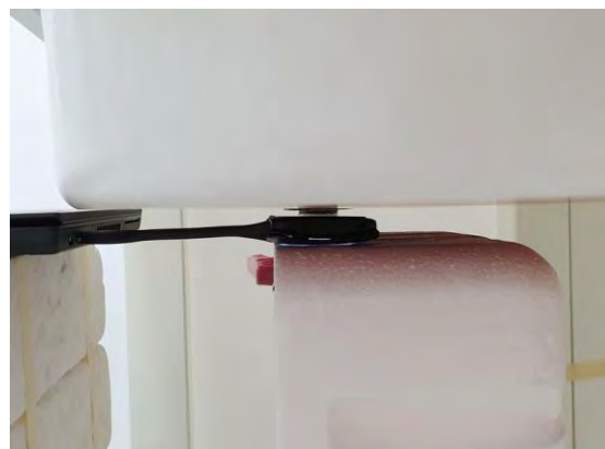
Fig.4 EUT Back side to flat phantom
