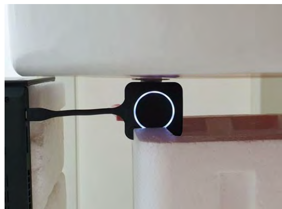
Fig.7 EUT Left side to flat phantom
