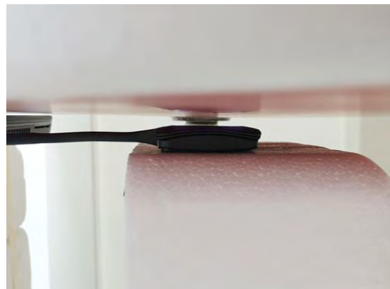
Fig.3 EUT Front side to flat phantom
