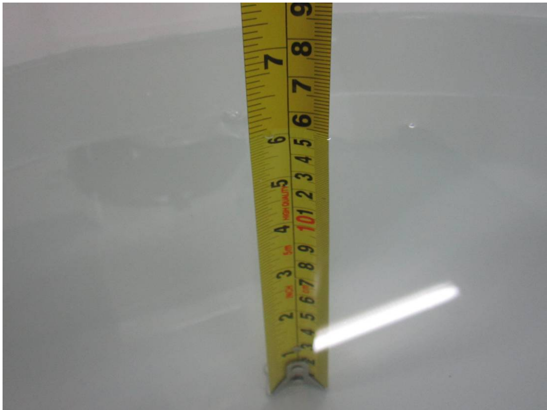
Liquid depth \geq 15\text{cm}
