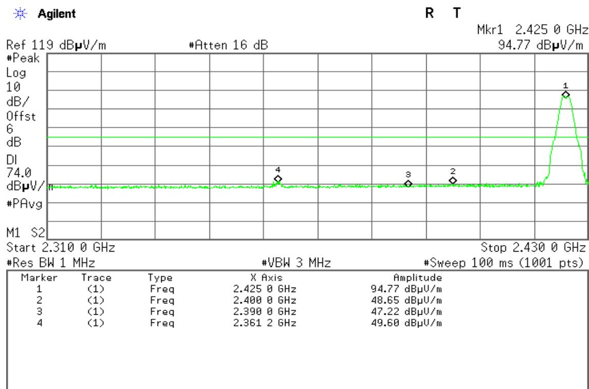
**Detector mode: Average****Polarity: Vertical**
