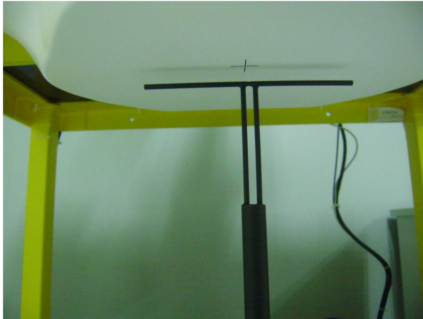
Setup Photo of Dipole Antenna
