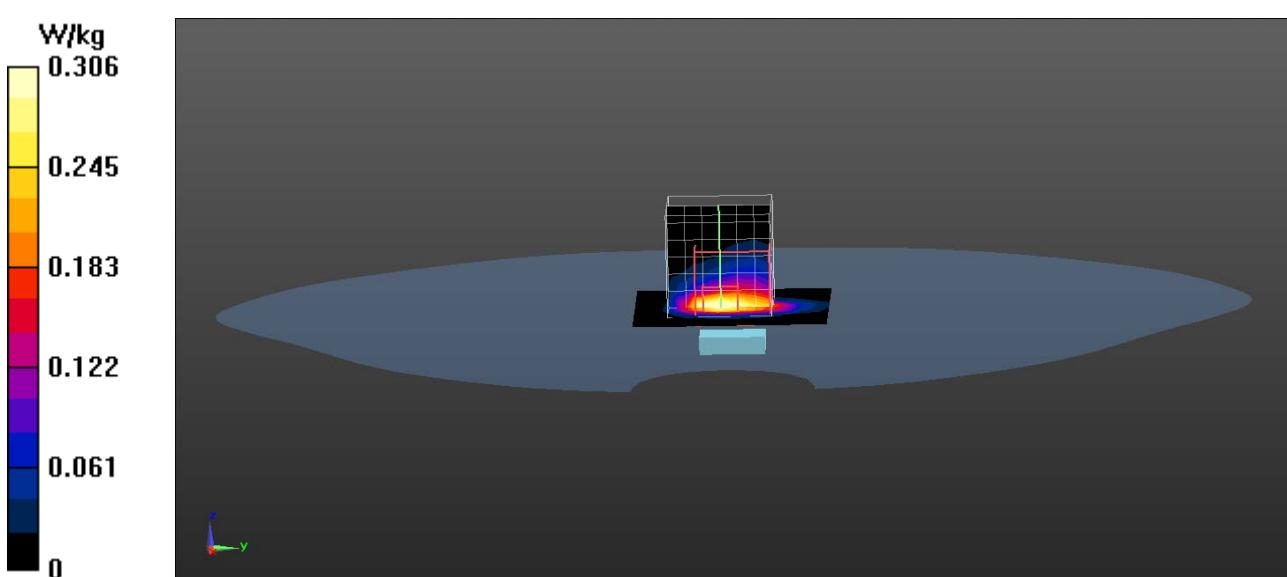
**802.11b EUT Back, Z-Axis plot****Channel: 11**
