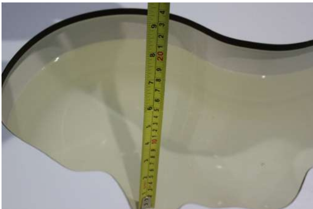
Picture 7-8: Liquid depth in the Head Phantom(5GHz)
