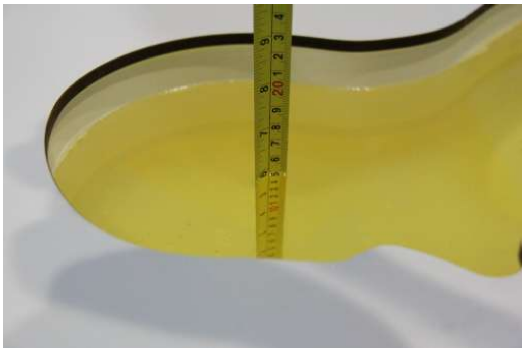
Picture 7-6: Liquid depth in the Head Phantom(2450MHz)
