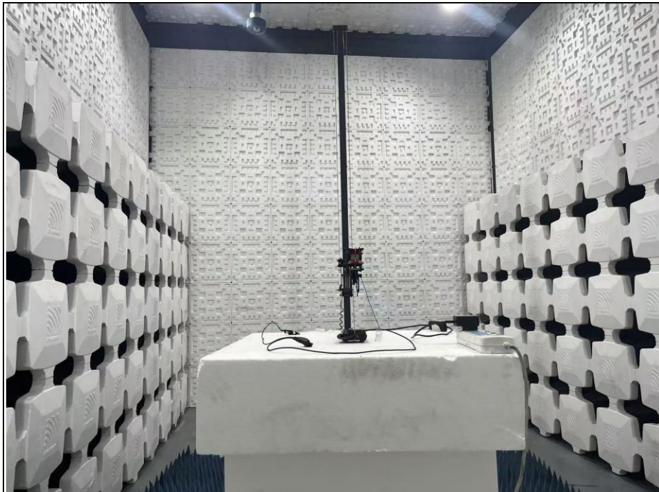
Radiated emission test: Frequency Range < Above 1GHz >
