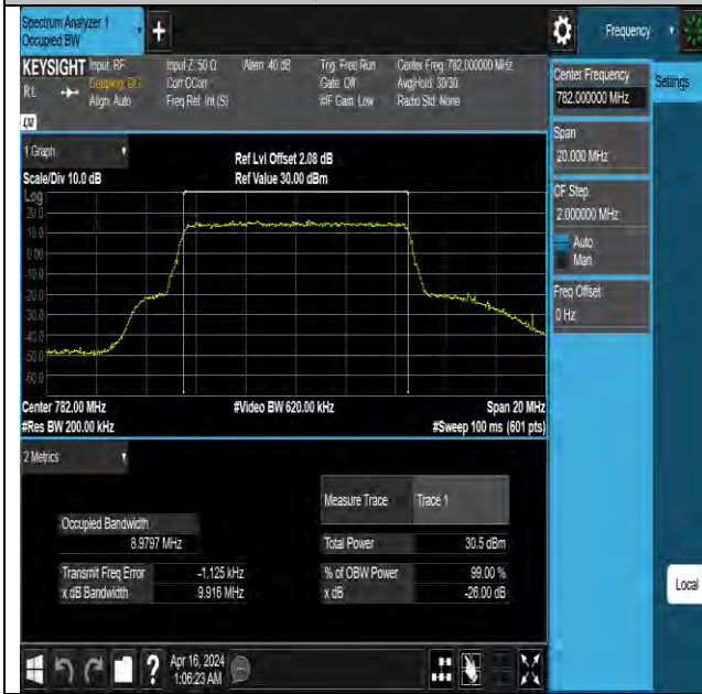
Band13-10MHz-QPSK-23230-50RB#0-PASS
