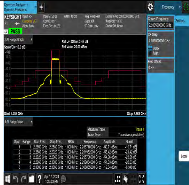
Band30 5MHz QPSK 27735 25RB#0
