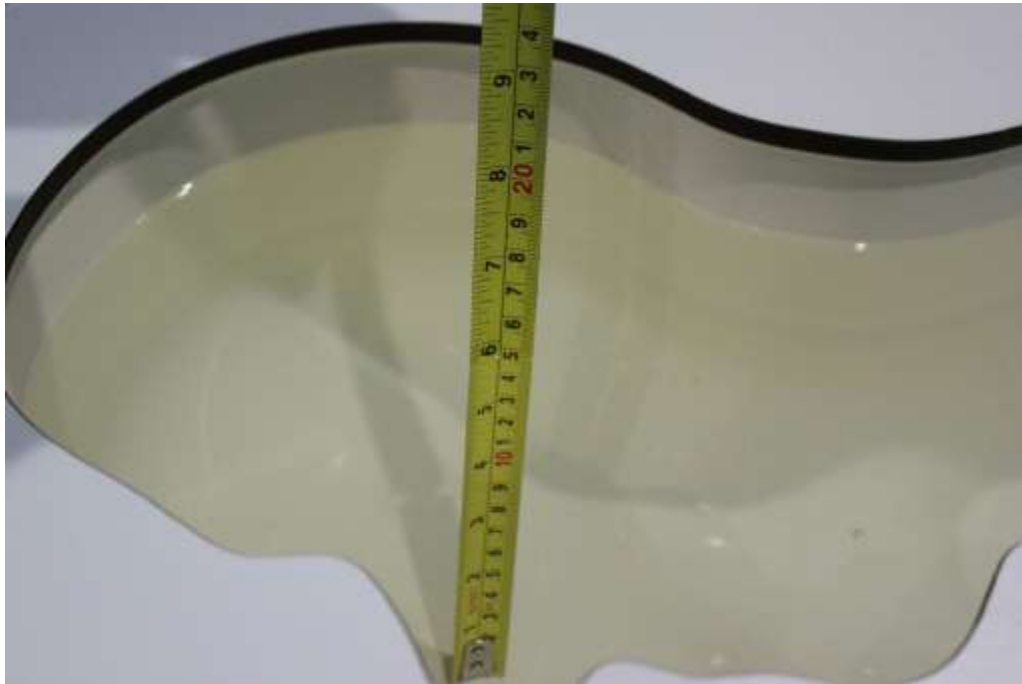
Picture 7-7: Liquid depth in the Head Phantom(5GHz)
