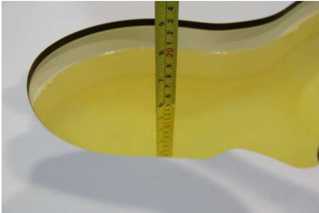
Picture 7-5: Liquid depth in the Head Phantom(2450MHz)
