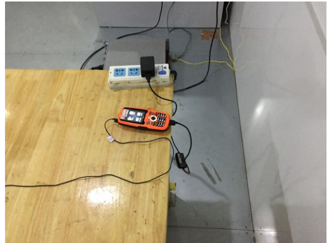
Conducted Emissions Test Setup – Side View
