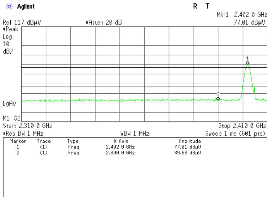
**Detector mode: Average****Polarity: Vertical**
