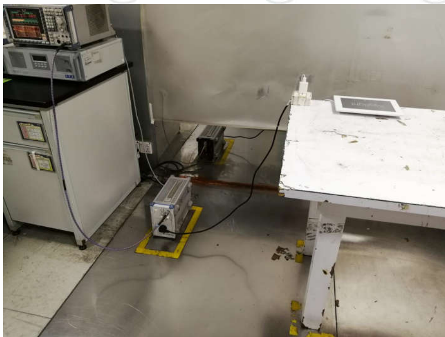
Conducted Emissions Test Setup
