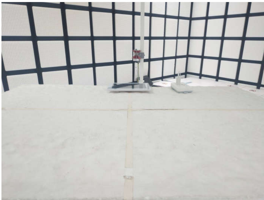
Radiated spurious emission Test Setup-2(Above 1GHz)
