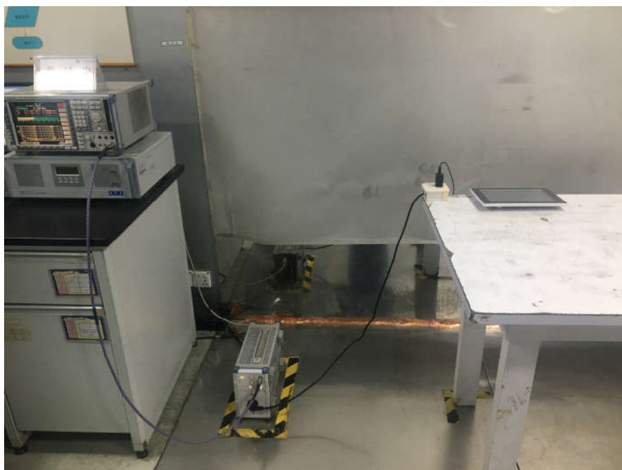
Conducted Emissions Test Setup
