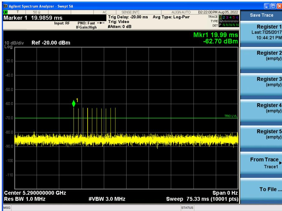
Radar Type 0 (80MHz / 5530MHz)
