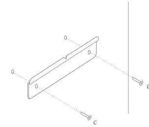
2. Align the pleat with the grooves located at the back of the device, near the top, and hook the device on.
