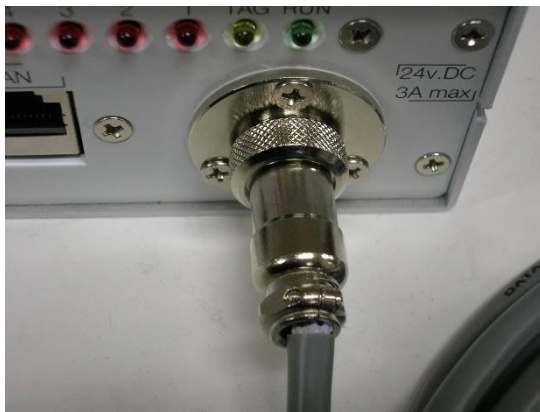
(1) Connection Power connector of Reader with connector of SMPS cable
