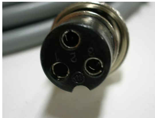
(1) Connection Power connector of Reader with connector of SMPS cable
