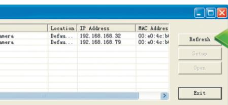
The router automatically gives your camera an IP address. If not, click **“refresh”** till it shows up. Double Click the IP address to run the camera. You'll see:
