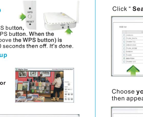
Press the camera **WPS** button, then press router's **WPS** button. When the camera's blue light(above the **WPS** button) is continuously on for 10 seconds then off. It's done.
