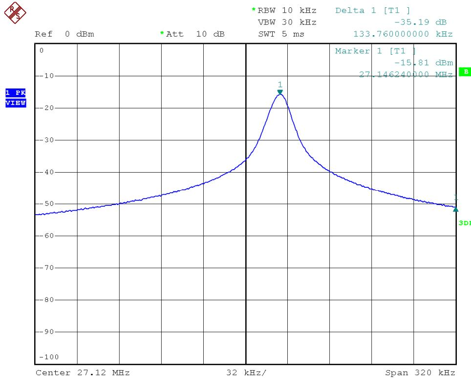
Bandwidth / Bandedge-Plot – Pursuant to FCC Part 15 Section 15. 227 Requirement (Pass/Fail)
