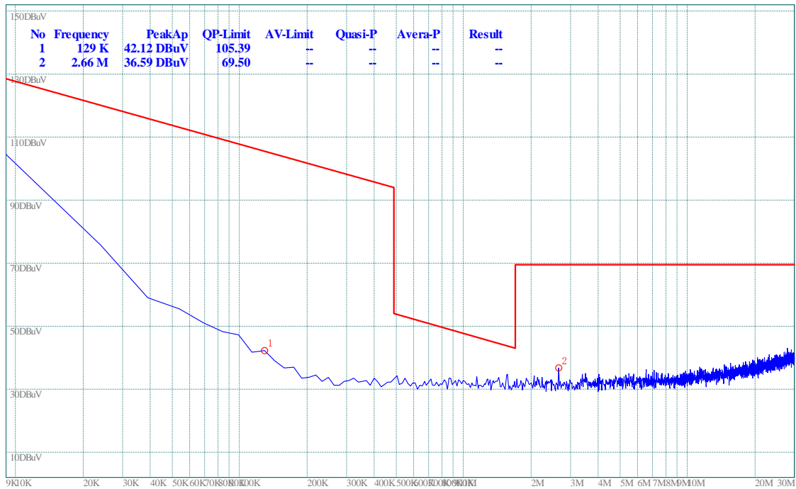
(Plot B.0: 9kHz to 30MHz @ GFSK, channel 39)
