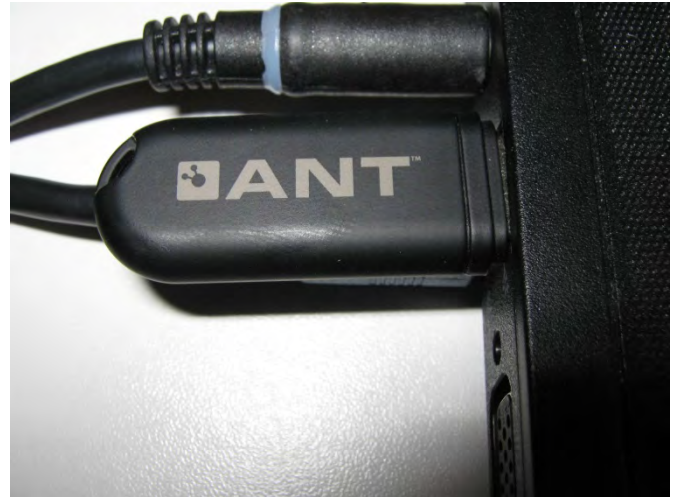
Photograph 2.3-2: ANT USB2 Stick plugged into Laptop PC
