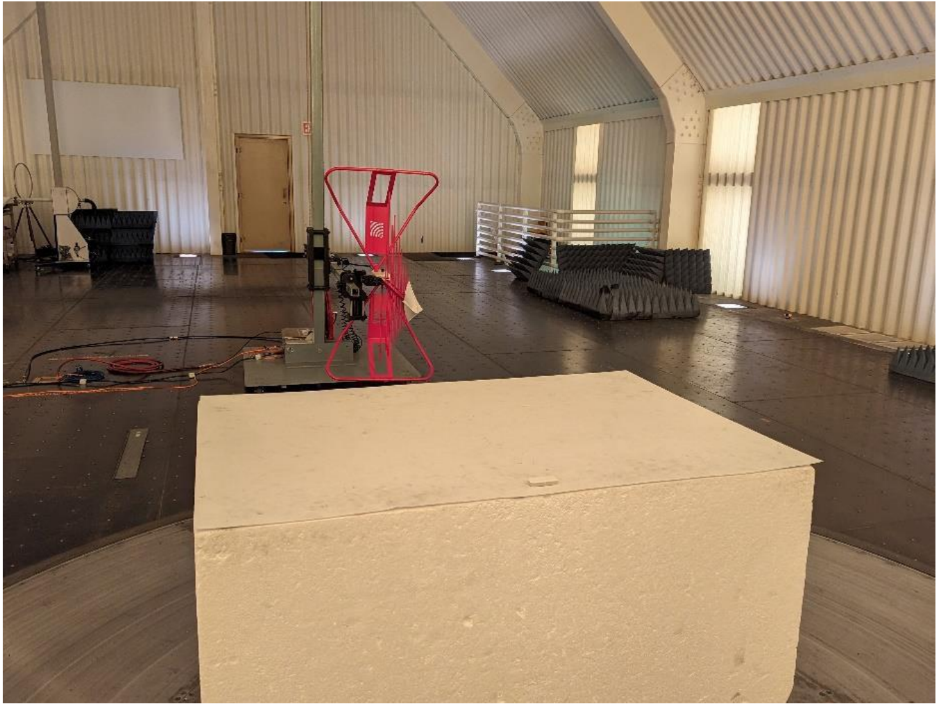
Photograph 2: Back View Radiated Emissions Worst Case Configuration
