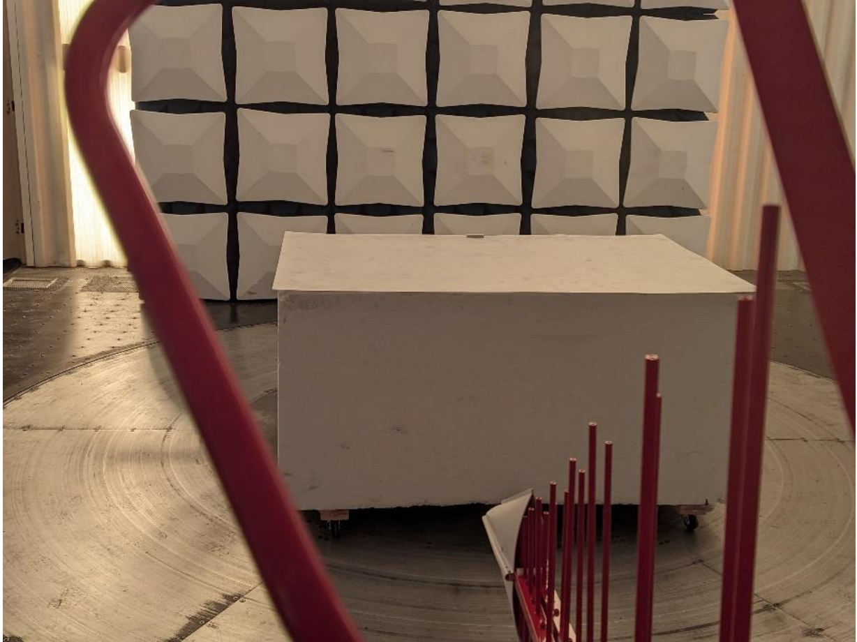
Photograph 1: Front View Radiated Emissions Worst Case Configuration
