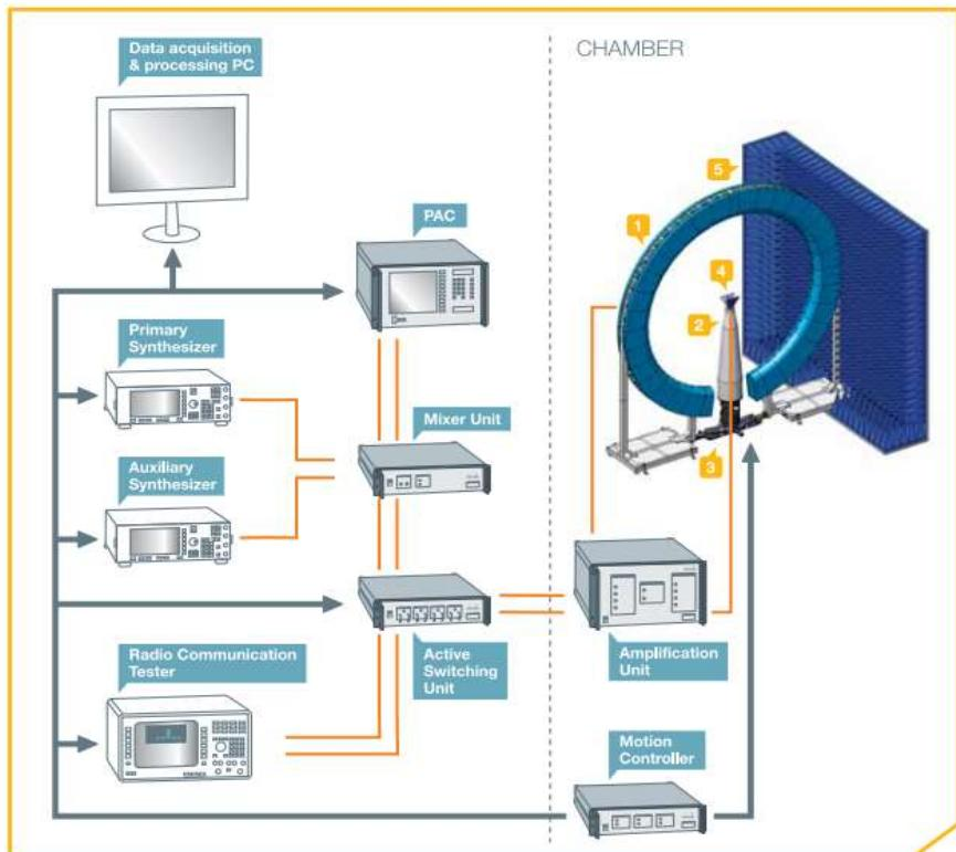
SG 64 uses analog RF signal generators to emit EM waves from the probe array to the antenna under test (AUT) or vice versa.
