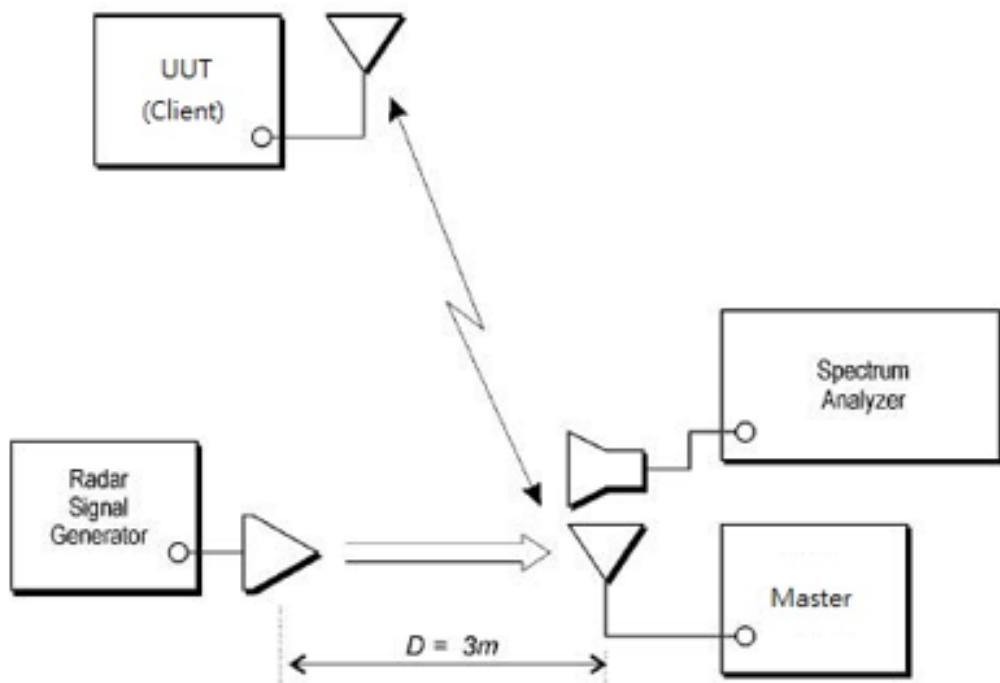
The UUT is a U-NII Device operating in Client mode without radar detection. The radar test signals are injected into the Master Device. Applicable Evaluation Criteria
