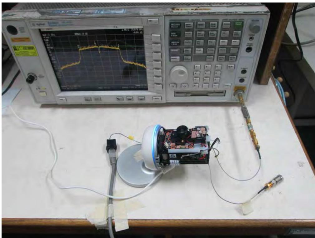
**RADIATED EMISSION SETUP****Below 1GHz**
