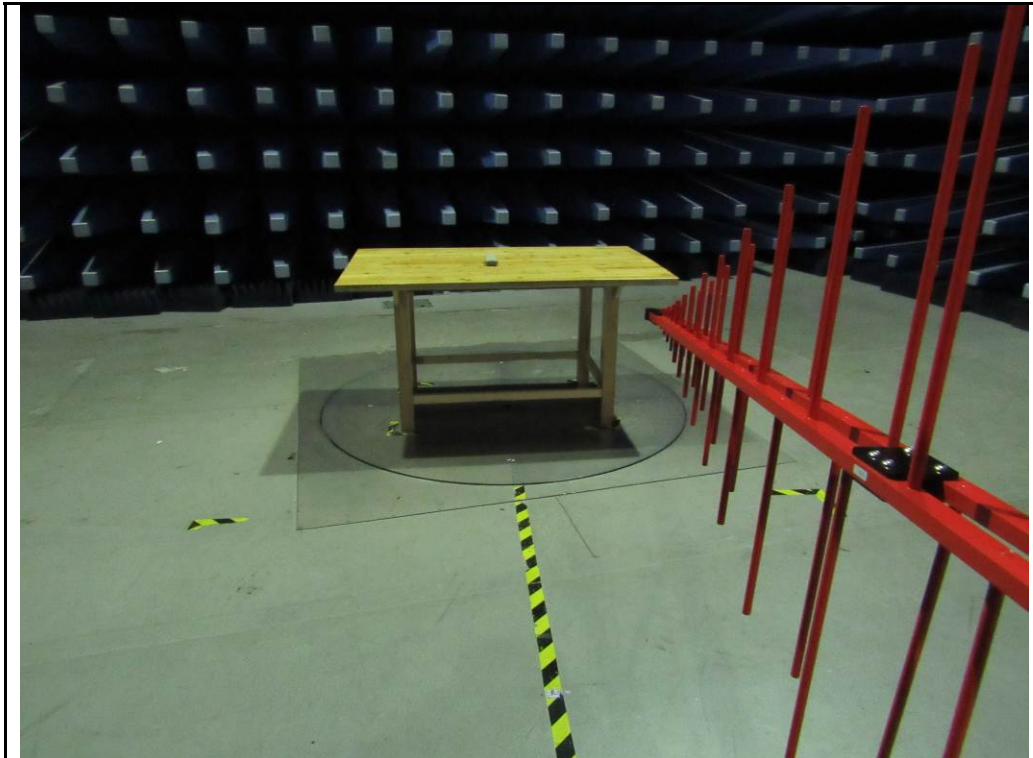
Radiated Spurious Emissions Test Setup Below 1GHz
