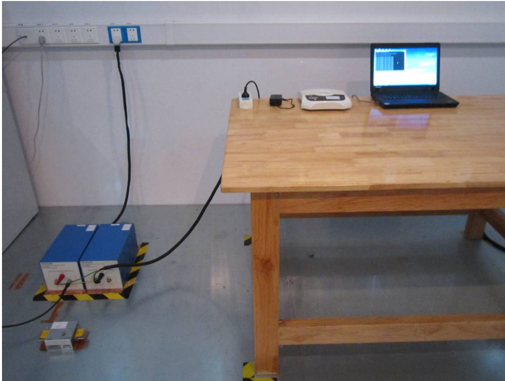
Conducted Emissions Test Setup Front View
