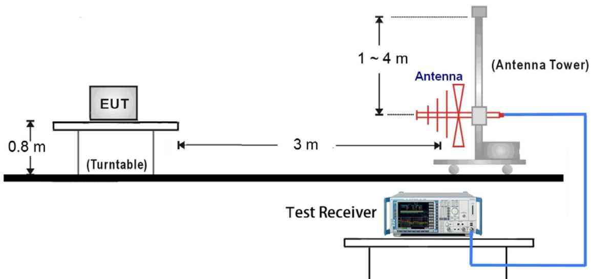
1GHz ~ 25GHz Test Setup:
