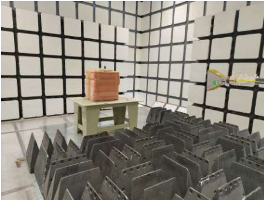
Radiated Emissions View (Above 1 GHz)
