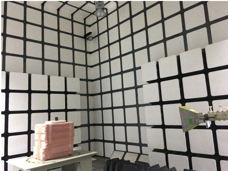
Radiated Emissions View (Above 1 GHz)
