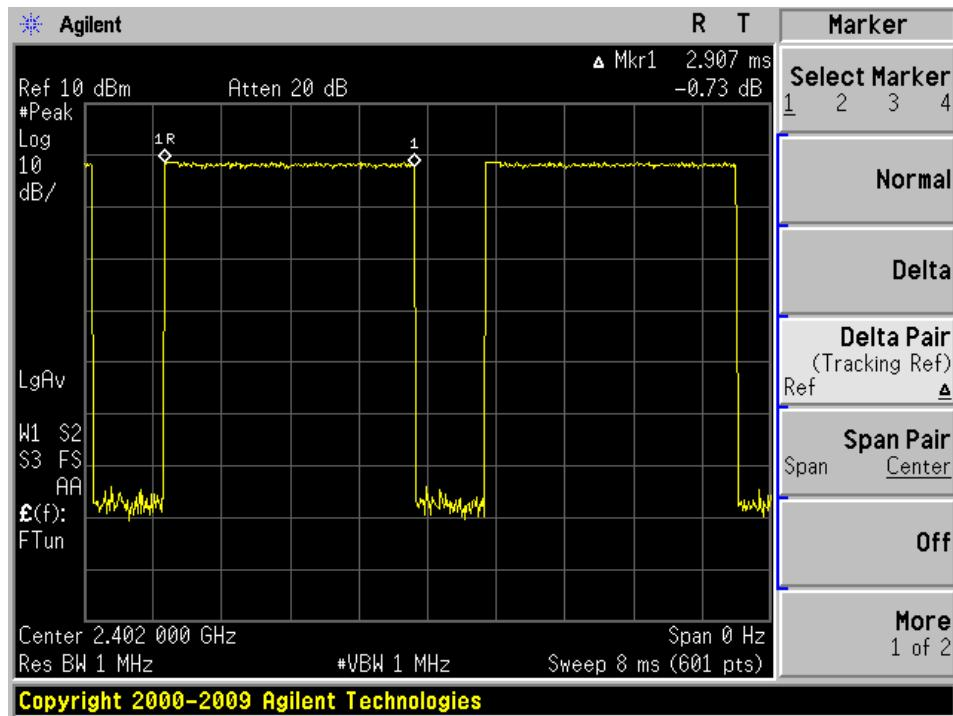
Result data graph shows the pulses duration of DH3 Package at 3MHz
