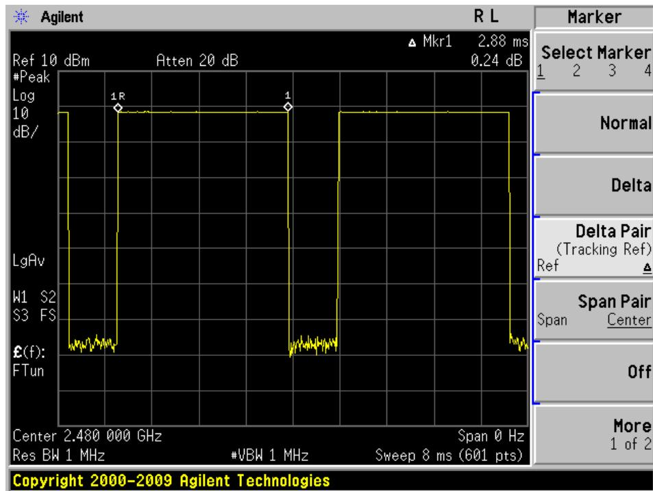
Result data graph shows the pulses duration of DH3 Package at 1MHz
