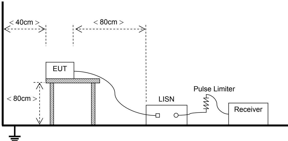
The EUT is placed on a 0.8m high insulating table, which stands on the grounded conducting floor, and keeps 0.4m away from the grounded conducting wall. The EUT is connected to the power mains through a LISN which provides  $50\Omega/50\mu\text{H}$  of coupling impedance for the measuring instrument. A Pulse Limiter is used to protect the measuring instrument. The factors of the whole test system are calibrated to correct the reading.
