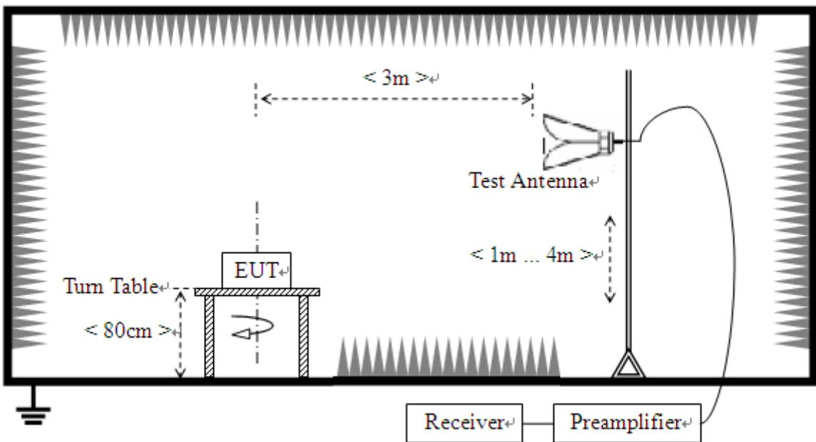
The test is performed in a 3m Semi-Anechoic Chamber; the antenna factor, cable loss and so on of the site (factors) is calculated to correct the reading. The EUT is placed on a 0.8m high insulating Turn Table,
