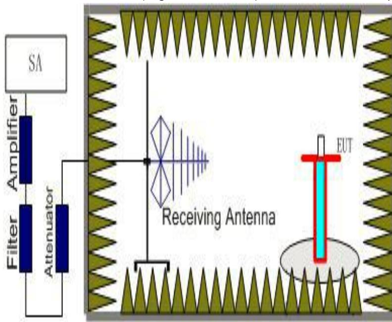
2. The EUT is then put into continuously transmitting mode at its maximum power level during the test. And the maximum value of the receiver should be recorded as (Pr).
