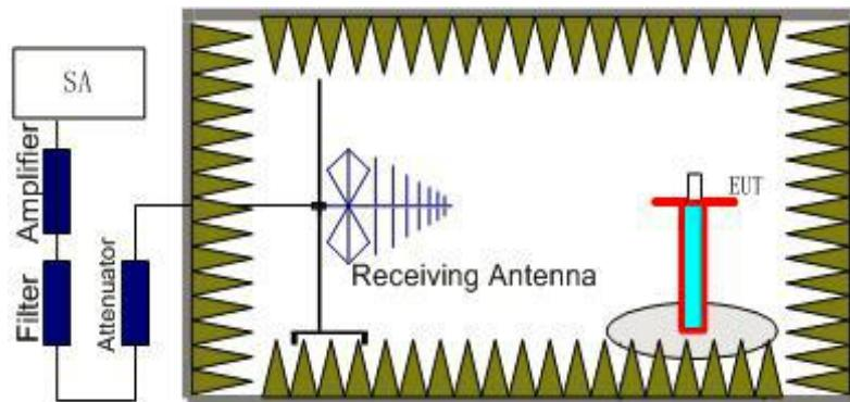
2. The EUT is then put into continuously transmitting mode at its maximum power level during the test. And the maximum value of the receiver should be recorded as (Pr).
