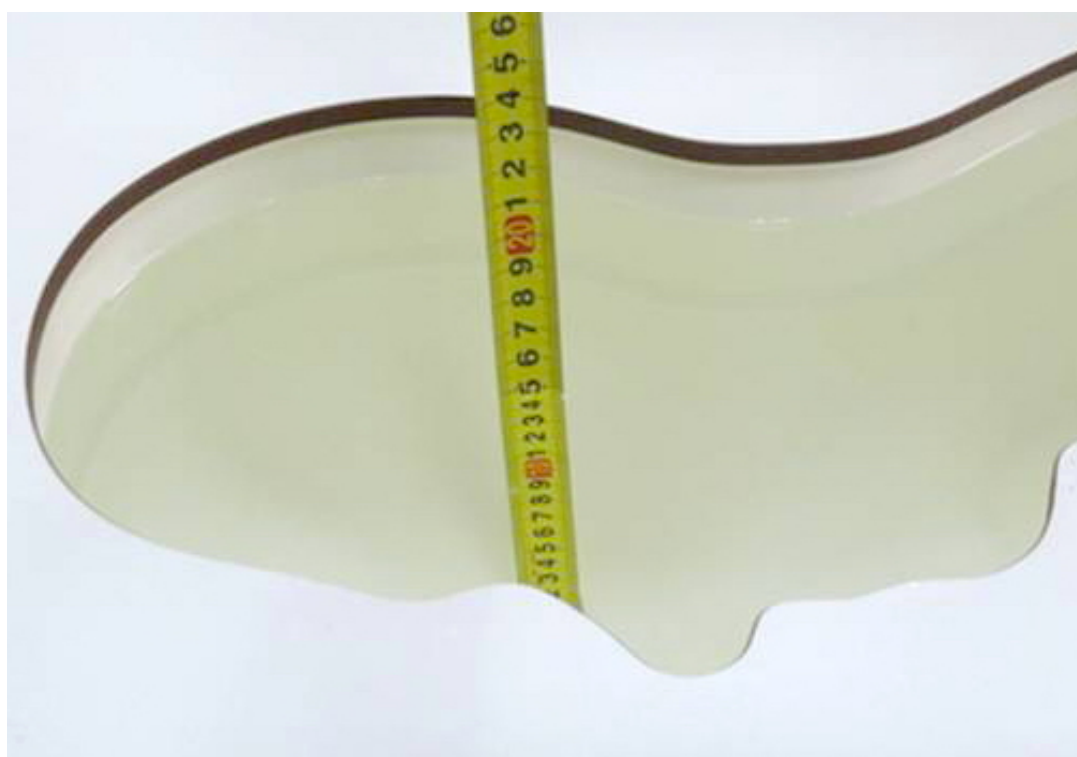
Picture 3: liquid depth in the head Phantom (1750 MHz, 15.3cm depth)
