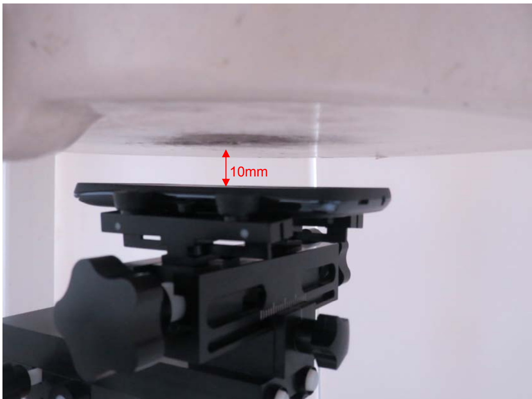
Picture 10: Front Side, the distance from handset to the bottom of the Phantom is 10mm
