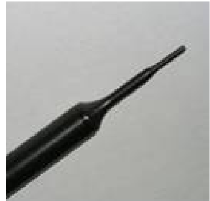
Figure 2. EX3DV4 E-field Probe
