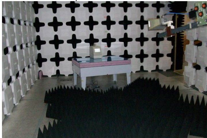
Antenna Setup: Horn Antenna – Above 1GHz
