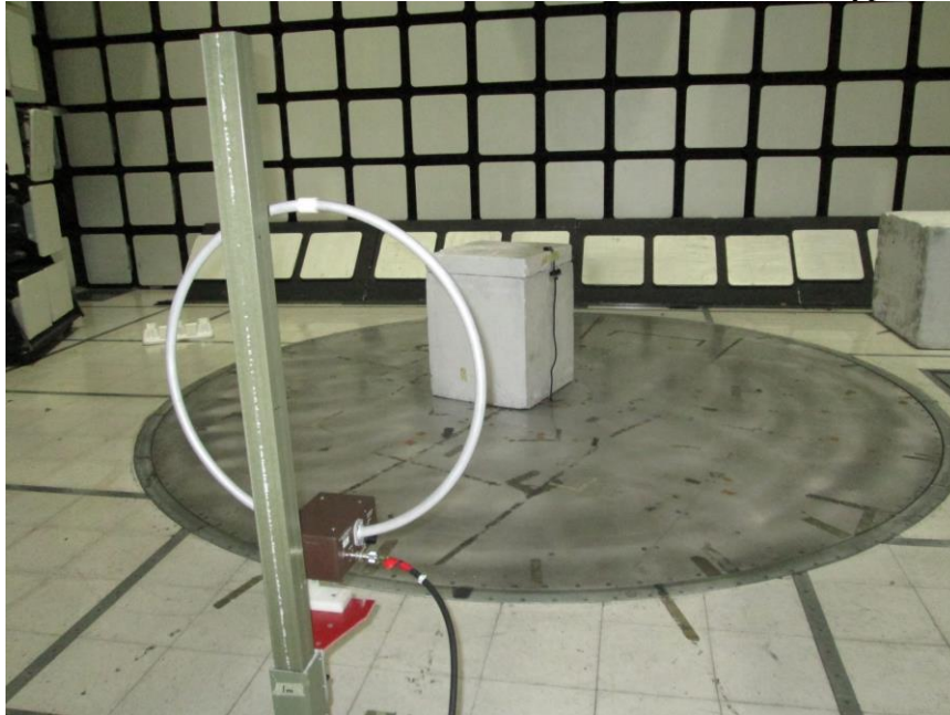
RADIATED PHOTO (9 kHz to 30 MHz) 10m – Dimmer2 and Bypass2
