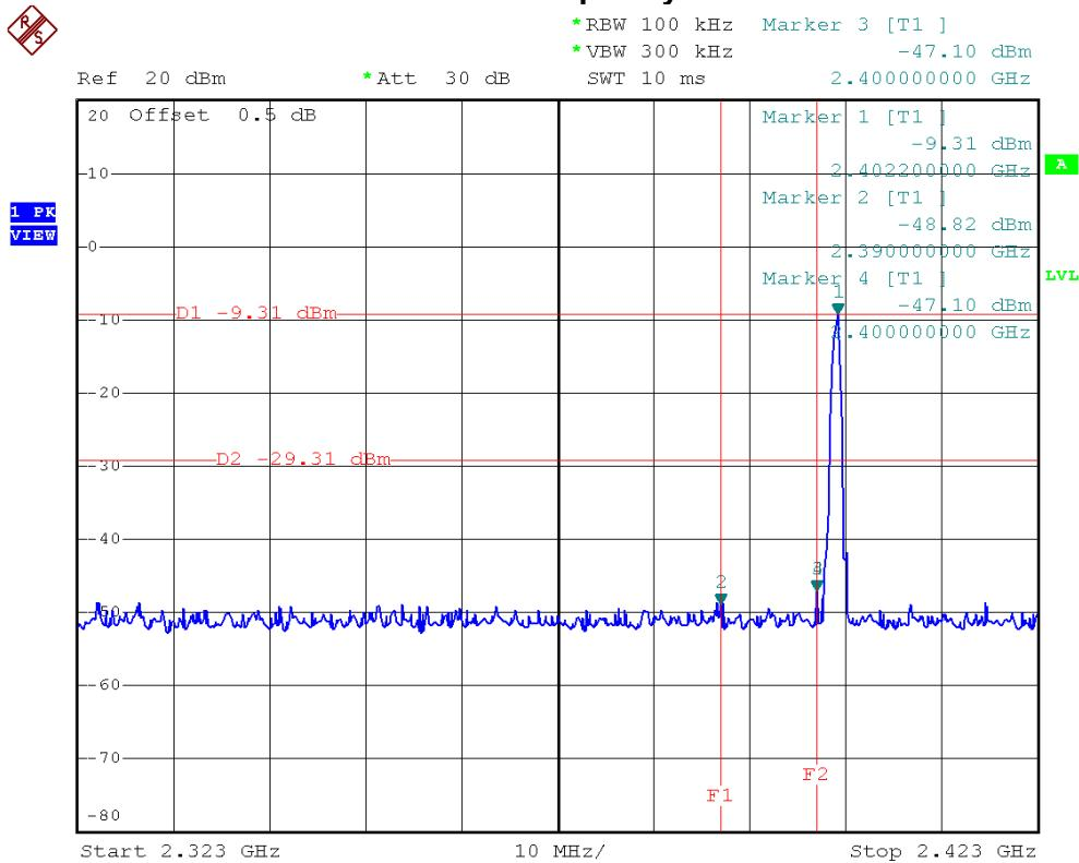
**The max. radio frequency power in any 100 kHz bandwidth within the frequency band**
