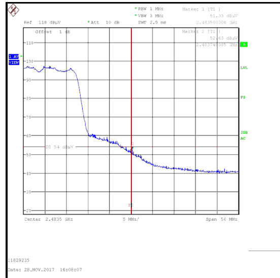
Upper Band Edge Average Measurement
