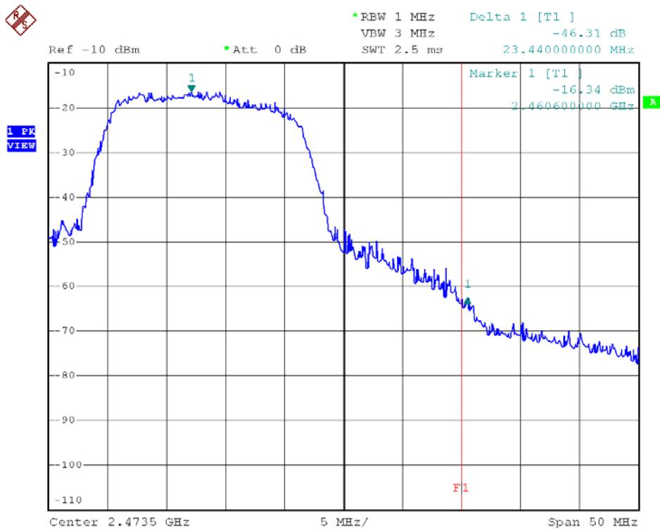
Bandwidth / Bandedge Plot – Pursuant to FCC Part 15 Section 15. 249 Requirement (Pass/Fail)
