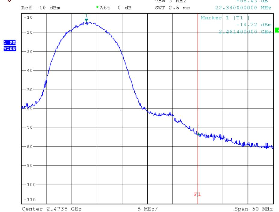
**Bandwidth / Bandedge Plot – Pursuant to FCC Part 15 Section 15. 249 Requirement (Pass/Fail)**
