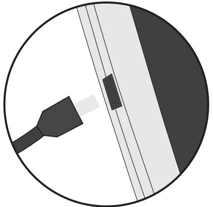
Charge your device by plugging your power cable into the micro-USB port. The snakebyte Vyper device will turn on and start charging. The charging indicator light is on when the battery is charging.
