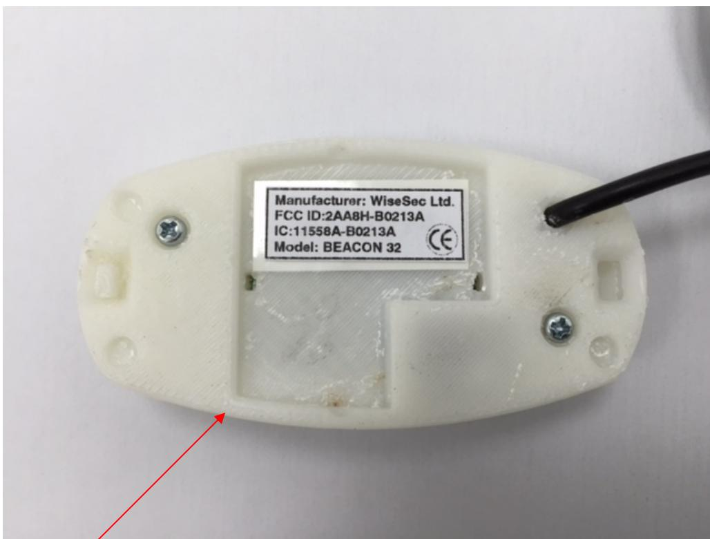
Label with **FCC ID:2AA8H-B0213A** is located at the rear side panel of the device. The statement according to FCC part 15 §15.19(a)(3) is placed in User's Guide, page 4 (Application exhibit User\_manual\_24511).
