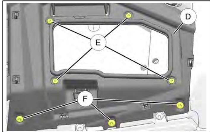
3. Tilt steering wheel down. Remove and retain four screws **E** from dashboard top **D**.
