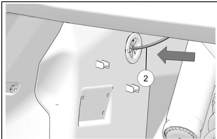
3. Route antenna harness ② along accessory mounting panel. Secure in tabs along edge of panel.
