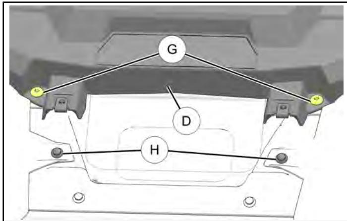
7. Carefully keep panels **J** and **K** up and away from tabs and remove dashboard top **D** by tilting rear section up and pulling out toward rear.
