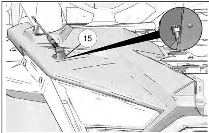
3. Pass antenna mount post ⑯ through ground strap ⑦, antenna harness ②, and secure with one nut ⑫. Place harness boot over nut after torquing.
