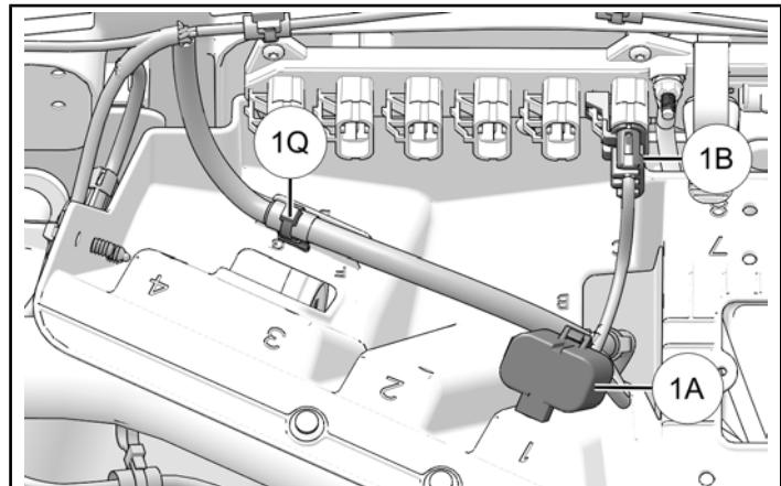
3. Route amplifier connector 1C and 1D through bottom opening of accessory mounting panel. Secure harness to accessory mounting panel with one routing edge clip 1Q. Join audio harness connectors 1C and 1D to amplifier.
