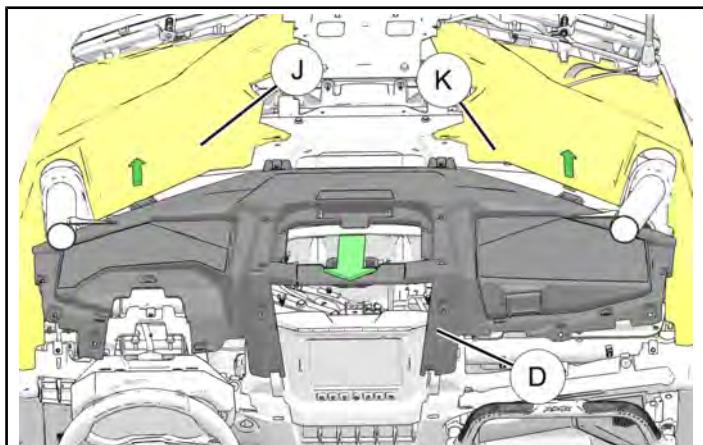
5. Carefully lift edge of left front fender **J** to release tab from dashboard top **D** as shown.
