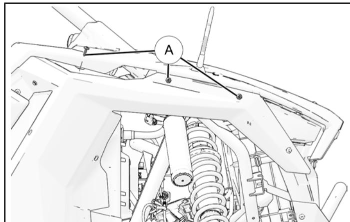
3. Reinstall hood nose panel with one fastener ④.
