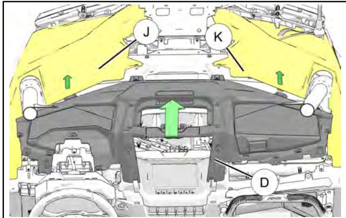
2. Ensure that tabs on panels ① and ⑩ are aligned in slots on dashboard top ④. (Only panel ⑩ shown. Panel ① is similar.)
