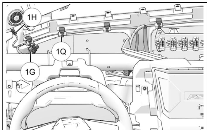
5. Join audio harness connector 1H to tweeter and connector 1G to driver.
