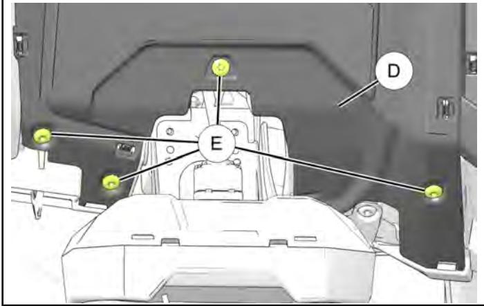
6. Open glove box lid. Install four retained screws **E** around glove box opening and three retained screws **F** in front of dashboard top **D**. Torque screws to specification.
