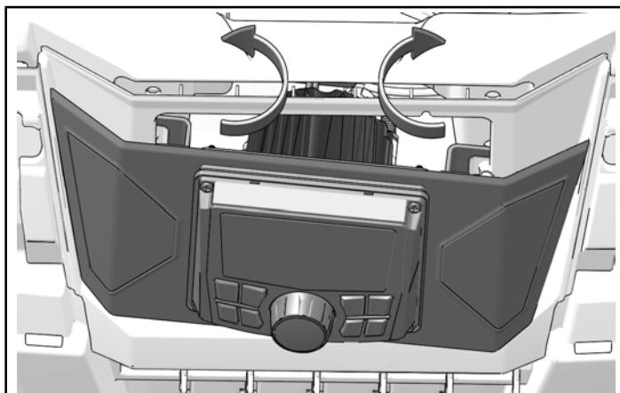
7. Secure PMX head unit to dashboard with four fasteners ⑩.
