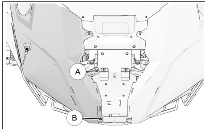
2. Reinstall right-hand hood panel with three hood fasteners Ⓐ.
