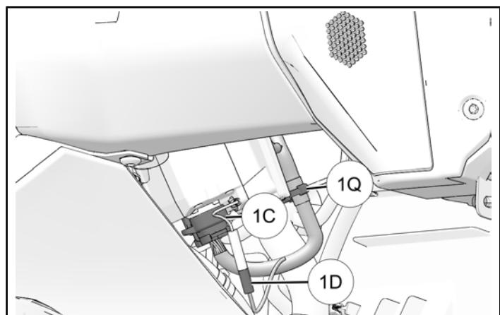
4. Route audio harness to driver side. Secure to front cab panel with four routing clips 1Q.
